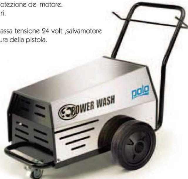
Professional cold water pressure cleaner with group pump motor at 1450 rpm, motor at double bearings and pump with three ceramic pistons, connecting rods and camshaft.
